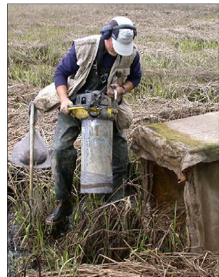
Figure 4-7. Vacuum for collecting insects, using a large-diameter tube (Credit: Fritz Grevstad, Oregon State University)
